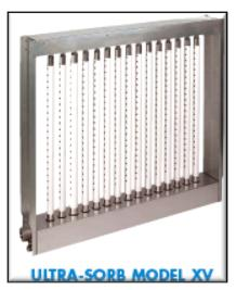
management system which is an industry first for pressurized steam. The XV design includes a secondary heat exchanger to vaporize any dispersion-generated condensate and also returns pressurized condensate to the boiler without additional pumps, valves, vents, or controls. There is zero water waste - all condensate returns to the boiler while still hot, saving energy, water, and boiler chemicals.
